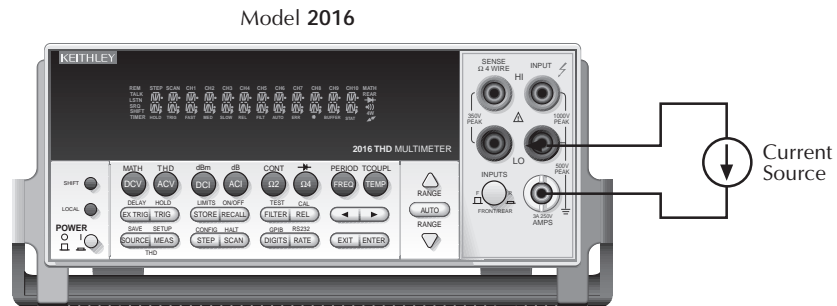
Figure 2-5 DC and AC current measurements
